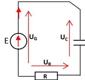
$\frac{du}{dt} + \frac{1}{RC}u = \frac{E}{RC}$  on tire  $a = \frac{1}{RC}$  et  $b = \frac{E}{RC}$
